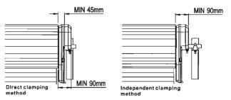
Ensure that there is at least 45 mm from the edge of the curtain to the edge of the bracket. If the roller door drum is on the edge of the curtain or is a smaller diameter, additional clearance may be required.
